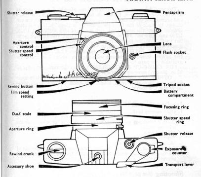
The Mamiya Sekor 528TL is a much simplified version of the TL models, its lens is fixed but tele and wide-angle attachments are available. The shutter is a between-lens type with speeds from 1/15 to 1/500 sec. The meter reads through the lens and has a manual override. The flash contact is in the accessory shoe on the pentaprism.
