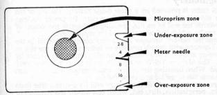
The aperture selected by the exposure meter is indicated by the needle position in the viewfinder. When the needle appears in the under-exposed zone, there is insufficient light for the speed of the film. When it appears in the over-exposed zone, the light is too strong for the film.
