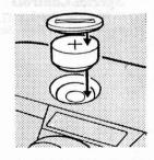
To change the exposure meter battery, unscrew the compartment cover with a coin and tip the old battery out. Insert the new battery with + side showing and replace the cover.
