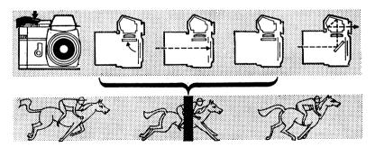
Below: When the shutter release is pressed, the iris diaphragm closes to the aperture pre-set, the mirror swings up and the shutter opens. When the shutter closes again, the mirror swings down and the iris diaphragm re-opens fully. While the mirror is in the upward position, the image cannot be seen, but this period is confined to that of the actual exposure, as signified by the black strip in the bottom diagram.
