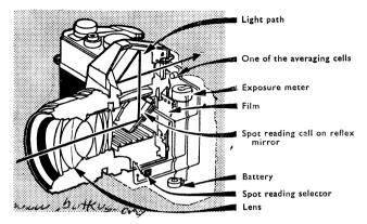
The image formed by the lens is reflected by the mirror on to the ground glass screen, whence it is again reflected to the eyepiece by the pentaprism. The image seen by the eye is right way up and right way round.
