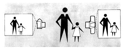
The viewfinder of the Mamiya Sekor shows the image upright and the right way round, whether the camera is held for horizontal (left) or vertical (right) shooting. With the standard lens the image also appears in approximately natural viewing size.
